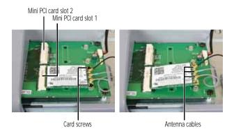
4 Slide the new card into an available card slot at a 30° angle, then press it down until the holes in the card line up with the screw holes in the case.
